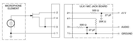
NOTE: LAVALIER MIC TIES PINS 3 AND 4 TOGETHER; THE GUITAR CABLE DOES NOT.
